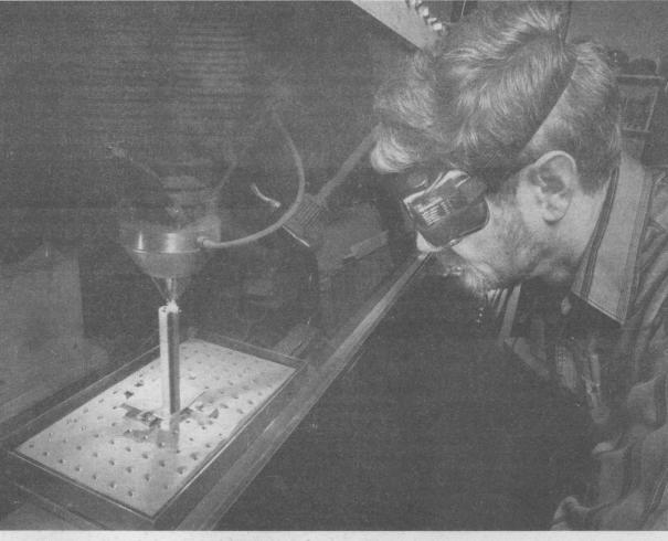
LASER SHAPING — Researcher Lane Harwell (1484) makes an 11-inch-high mini-skyscraper of the T-bird emblem using Sandia's Laser Engineered Net Shaping technique. Ten companies are teaming with Sandia in a two-year, \$3 million cooperative research and development agreement to commercialize the technology.
